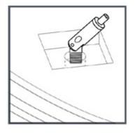
5. Press and hold the spring portion to insert the cable.
