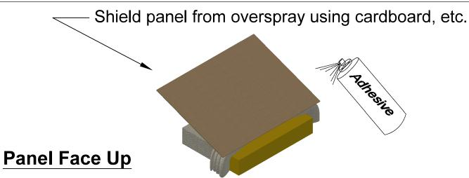
APPLY ADHESIVE TO EXPOSED PANEL CORE AND BACK OF FABRIC (ALL FIELD ALTERATIONS REQUIRE 1"FABRIC RETURN ON BACK OF PANEL)
