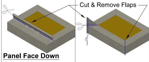
PINCH EXCESS FABRIC TOGETHER WITH FINGERS AND CUT OFF FLAPS WITH FABRIC SCISSORS
