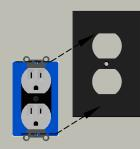
Remove outlet cover plate and pull outlet away from wall
