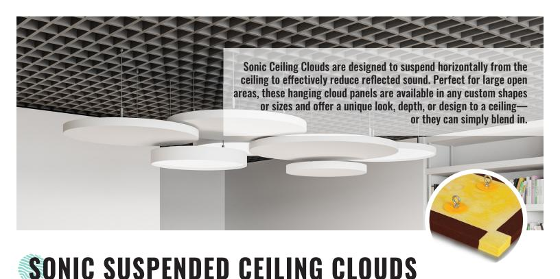
SONIC SUSPENDED CEILING CLOUDS core consists of a 6-7 lb. density rigid fiberglass board with resin hardened edges to reinforce panel perimeter against warping and damage. Your chosen finish selection is bonded directly to the panel face with all edges wrapped carefully and completely to the back of the panel to ensure a straight, flat, wrinklefree surface with tailored corners.
