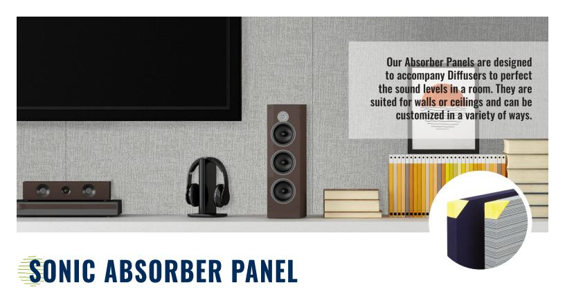
SONIC ABSORBER PANELS core consists of a 6-7 lb. density rigid fiberglass board layered with a 1/8" high density 10-20 lb. fiberglass sheet for added strength and tackability. Resin hardened edges to reinforce panel perimeter against warping and damage. Your chosen finish selection is bonded directly to the panel face with all edges wrapped carefully and completely to the back of the panel to ensure a straight, flat, wrinkle-free surface with tailored corners.
